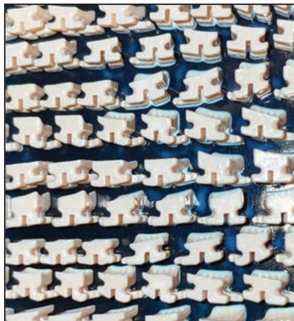
Fig. 1 LightForce* three-dimensionally printed brackets shown on printer build plate prior to processing.
